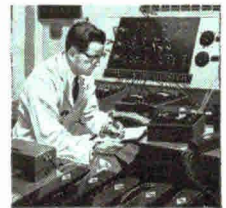
CBM Ballasts are checked by tests regularly, at E.T.L.
