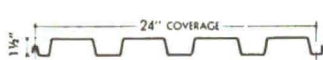
B-DECK —For spans to 10'0". Wide rib distributes metal for greater structural efficiency. Well suited for use as side wall panels.
