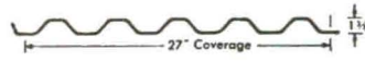
RIBFORM — High-tensile steel form for concrete slabs over spans up to 8'0". Three types: Standard, Heavy-Duty, Super-Duty (shown).
