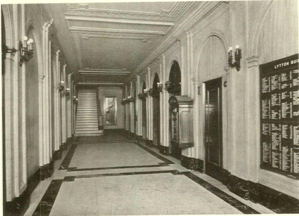
Entrance to Lytton Building, Chicago, Illinois. Architects, Marshall and Fox. Marble contractors, Henry Marble Company, Chicago, Illinois. Floor marble White Alabama and Verde-Antique border. Wall marble sunken panels, Alabama Pocahontas; remainder of wall marble above Verde-Antique base. Selected Alabama Cream A. Alabama marble furnished, finished and ready to set by the Alabama Marble Company.
