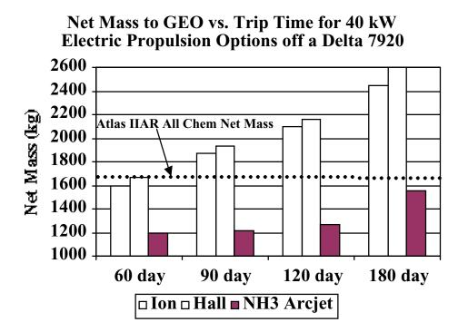
Figure 8.—Net Mass to GEO for 40 kW Hall Systems.
