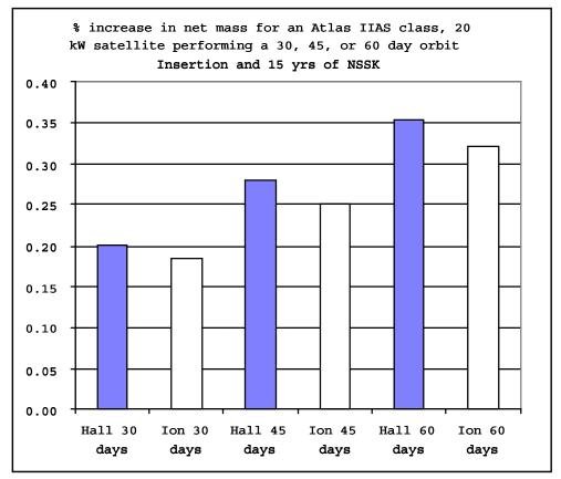
Figure 6.—GEO Payload Advantages with Hall Technology.
