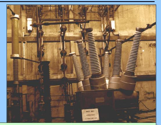
SYNTHETIC TESTS : Example of circuit-breaker under tests
