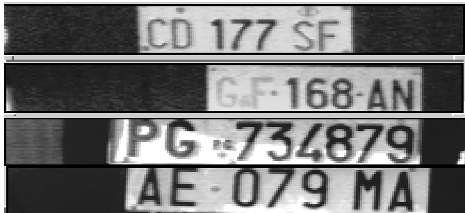
Fig. 7 Several images with multimodal histograms. In the case of the first two images, the plate has characters of two colours. The other two plates have strong shadows. All images have already been enhanced by stretching the histogram.
