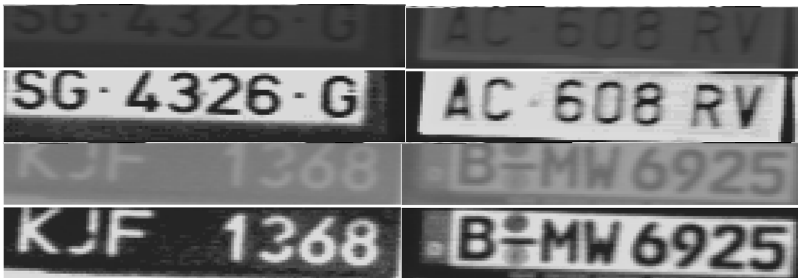
Fig. 4 Some processing of 4 interest areas. The first image in each group shows the interest zone in the original image (resampled). The second one shows the same area after histogram analysis and enhancement.
