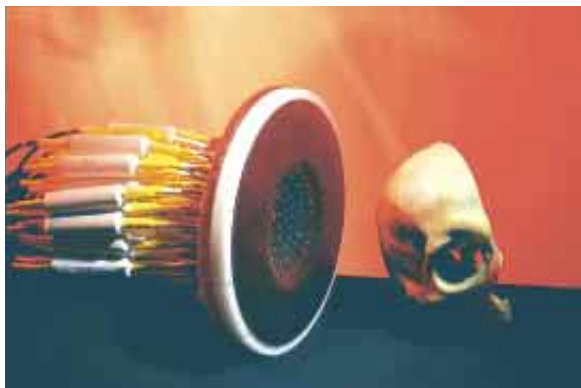
POROUS BONE IN THE SKULL presents an energy-sapping challenge to focusing ultrasound waves on a brain tumor to heat and destroy it. A time-reversal mirror with a modified playback algorithm can nonetheless focus ultrasound through skull bone onto a small target.
