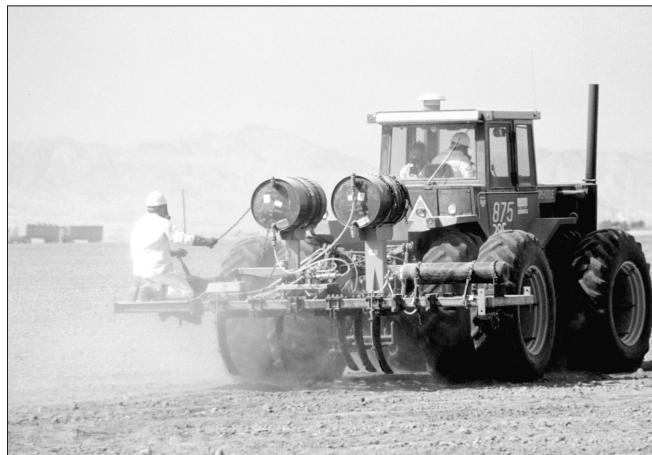
Telone is applied by shank injection into bare soil. In the left photo, the shanks are visible below the barrels. In the right photo, the shanks are underground, dispensing Telone.
