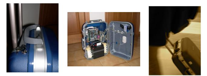
Apparently a simple trolley, the BlueBag contained a surveying system able to identify Bluetooth devices present in a 150 mt range.
