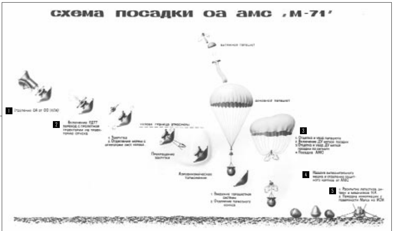
Figure 11. Enlarged Diagram of the Landing of the Automatic Martian Station of Mars 3— (1) orbiter and lander separation, (2) ignition of the solid propellant engine and transfer of the lander from the flyby to a Martian encounter trajectory, (3) ignition of the soft landing engine and separation of the engine with the parachute from the automatic Martian station plus withdrawal of the parachute, (4) landing of the automatic Martian station, inflation of the displacing bag, and separation of the aeroshell cover, and (5) opening of the petals, antennas, and mechanisms, initiation of the deployment of scientific instruments on the Martian surface, and transmittal of information to the Martian satellite
