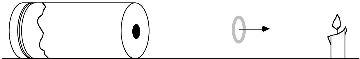
Figure 3.14 A device for producing smoke rings. The ring is stable and can blow out a candle several feet away.
