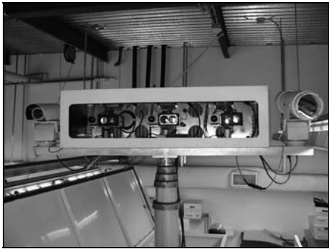
Figure 9. Mast top complete with rangefinders; view of mast inside van
