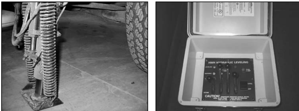
Figure 13. One leveling system jack and the leveling system controls
