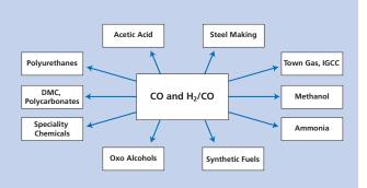
Remarkably, the right side of the diagram points to large quantities of syngas required to produce ammonia, methanol, synthetic fuels, for example.
