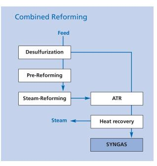
Generally, the feedstock contains impurities such as sulfur compounds to be removed because they would lead to downstream catalyst deactivation.
