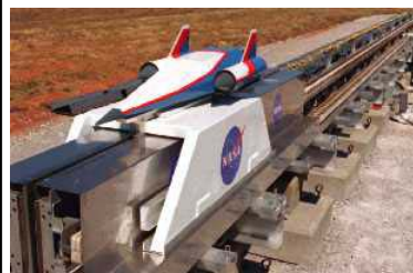
NASA Prototype aiming 300 m/s at 3g
