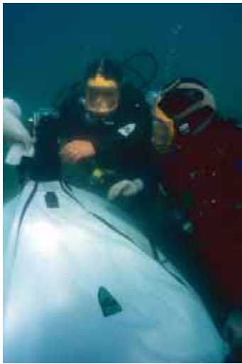
NPS researchers use an oil collection device to measure the quantity of oil seeping from the hull at different locations over a 24-hour period. NPS Photo by Brett Seymour
