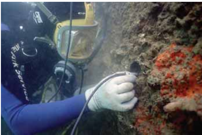
An NPS archeologist takes ultrasonic thickness measurements of the encrusted hull of the USS Arizona. NPS Photo by Brett Seymour
