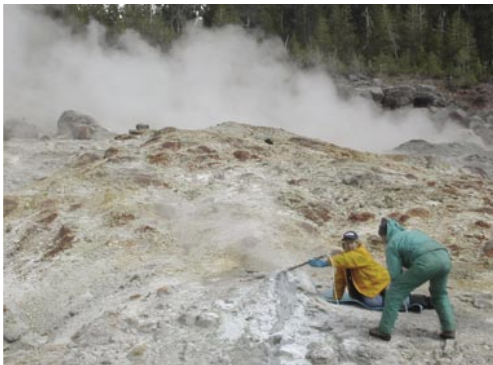
USGS volunteers Cathy Janik and Fraser Goff sample the gas from a fumarole on the flank of Steamboat Geyser.
