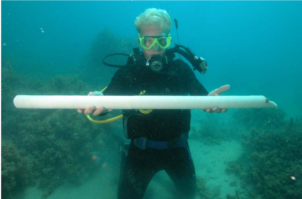
Core drilled from coral carbonate skeleton at Keswick Island, 33km offshore of Mackay.
