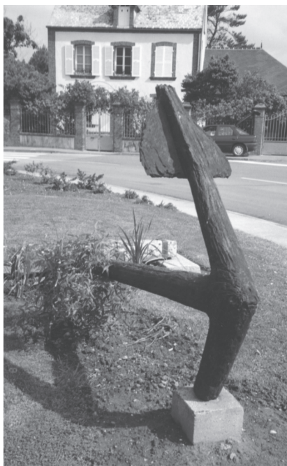
Figure 3. An ancient wrought iron anchor recovered from the sea. Note the wood-like appearance of the surface.
