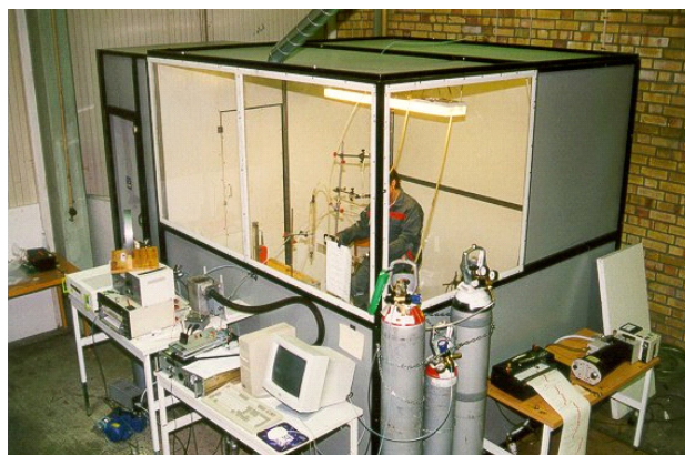
Figure 4. Exposure chamber for controlled exposure with diluted diesel exhaust.
