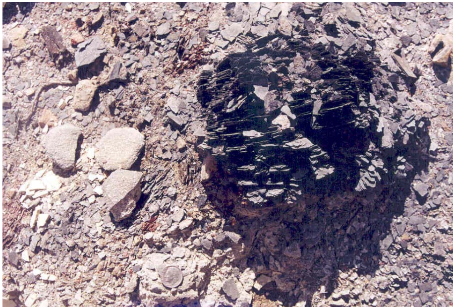
Figure 30. The Bobonaro Scaly Clay shows a high degree of fissility, which gives the clay a “scaly” appearance. A large variety of rock types occur as exotic blocks in this terane, which is spread over most of East Timor.
