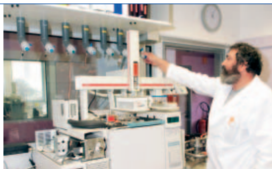
Head of Laboratory Vlado Kučan working with the gas chromatograph (r.). The gases are supplied via a dense network of pipes.
