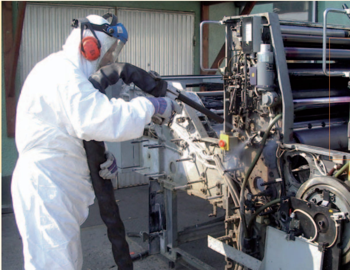
Putting the pressure on dirt: cleaning with dry ice.
