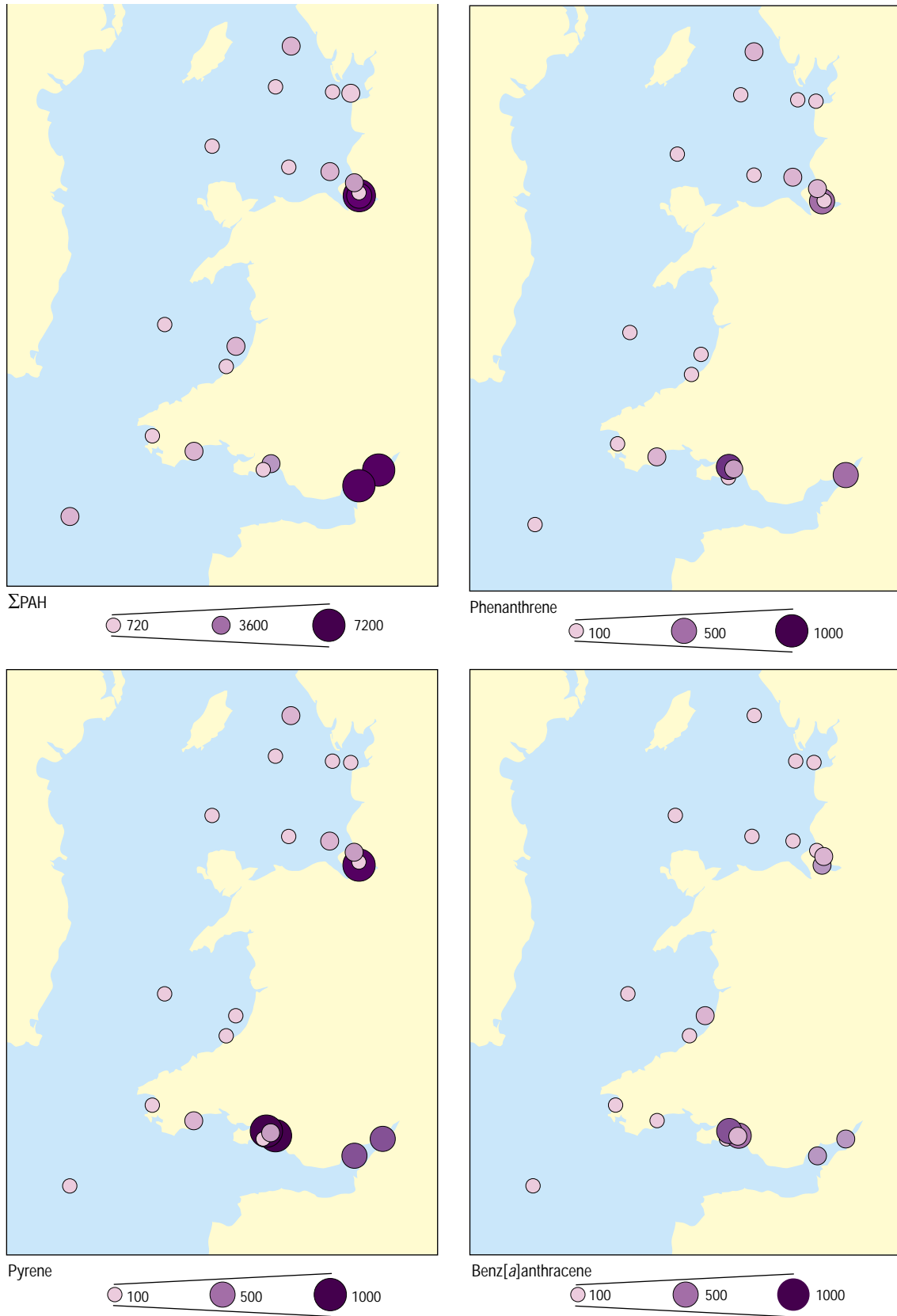
Figure 4.10 Polycyclic aromatic hydrocarbons in sediments ( \mu\text{g}/\text{kg} ) from the Irish Sea and Bristol Channel 1992–5. Source of data: CEFAS.
