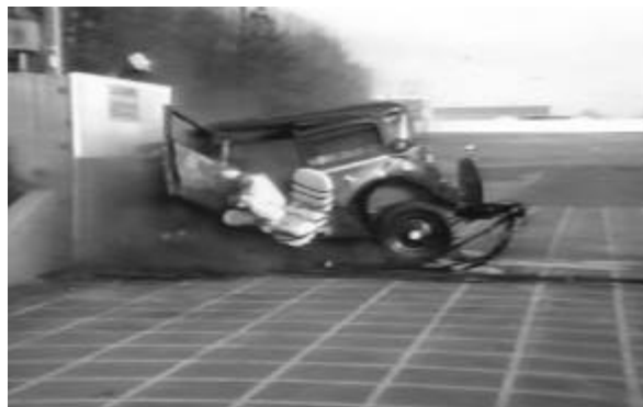
Figure 3: Crash Test of a 1929 Chevrolet with Unrestrained Occupants
