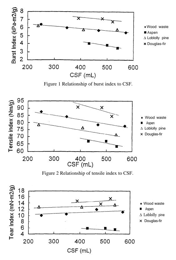
Figure 3 Relationship of tear index to CSF.
