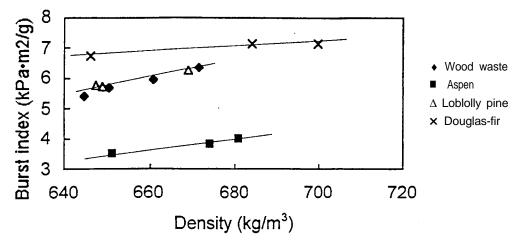
Figure 6 Relationship of density to burst index.
