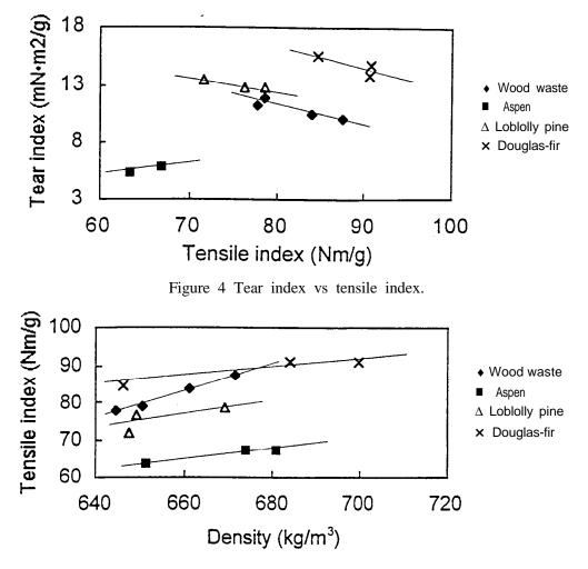
Figure 5 Relationship of density to tensile index.
