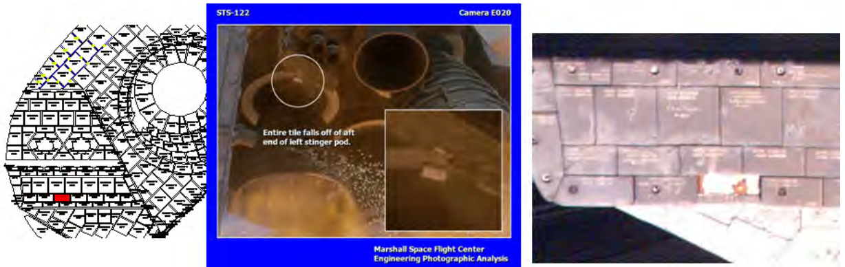
Figure 1 Location of the missing tile on the LOMS Stinger
