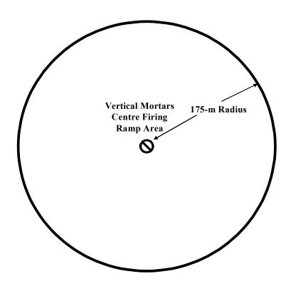
Figure 2. CIRCULAR SITE Vertical Mortars
