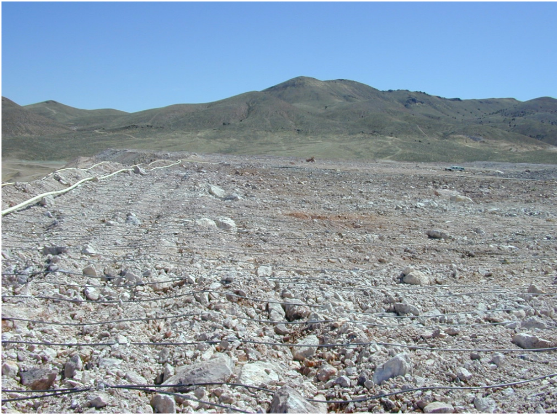
Figure 16.2 Brimstone Leach Pad and Recovery Pipes
