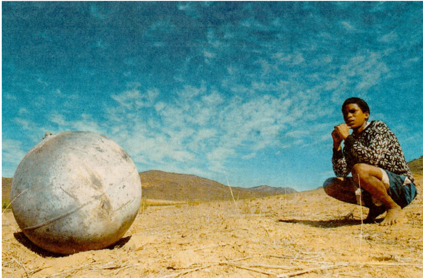
Figure shows a human-made pressurization sphere stemming from a rocket body that fell in Southern Africa
