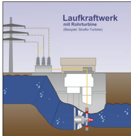
Figure 2.9: Run-of-river Power Station
