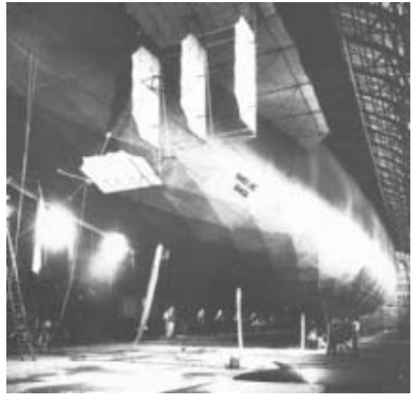
Fig. 4.40: View of drag inducing diamond pattern on the envelope of Schütte-Lanz airship SL-1. (Meyer 2 )
