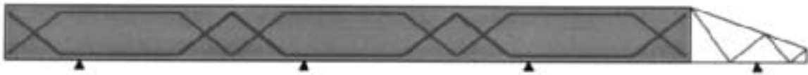
Fig. 4.34: Orientation of prestressing tendons in a launched prestressed concrete box girder bridge. (Vogel)
