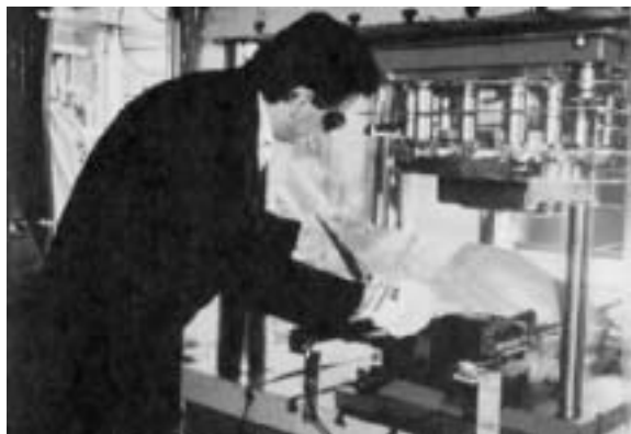
Fig. 6.4: Compression molding using thermoplastics and match cast metal dies. (Swanson)
