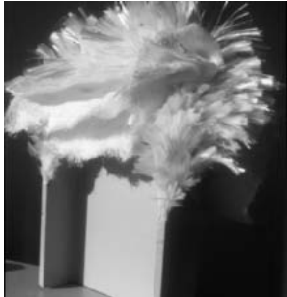
Fig. 3.9: Pultruded GFRP I-section with fiber mats showing. (CCLab)
