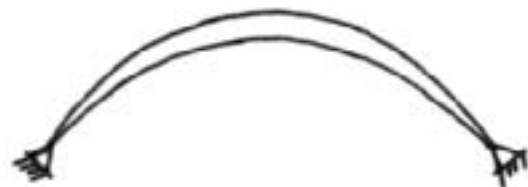
Fig. 3.4: Schematic of a two-hinge arch. (Dooley)
