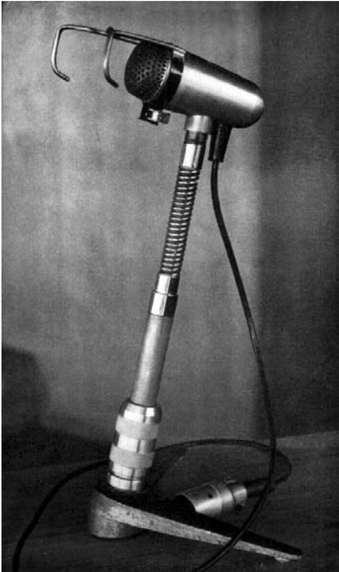
Lip microphone, designed and manufactured in Australia for the Games.
