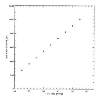
**Figure 5.** Flow rate versus channel runout distance for the Mars case.
