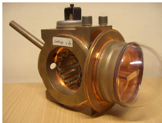
Figure 4.1: Image of an S band magnetron (e2v type MG5193)
