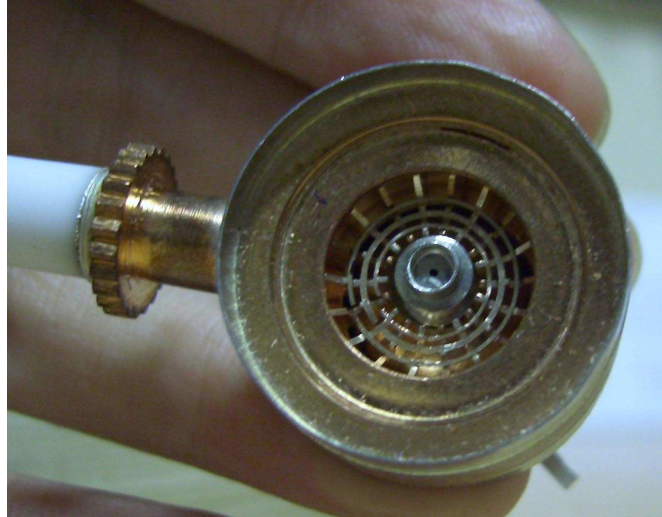
Figure 5.1: Image of an X band magnetron (e2v type MG5241)
