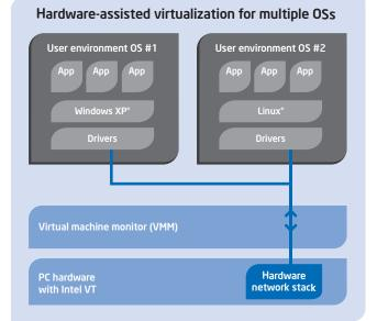
**Figure 7. Hardware-assisted virtualization.** Virtualization provides IT with isolated, secure spaces in which to abstract or stream OSs and applications. Both next-generation and traditional virtualization is supported on notebook and desktop PCs with Intel<sup>®</sup> vPro<sup>™</sup> technology.
