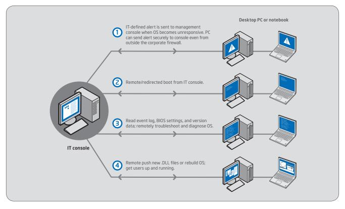
Figure 6. Remote problem resolution for an inoperable OS. The capabilities allow a technician to remotely access, diagnose, and repair or rebuild an OS that has become inoperable.
