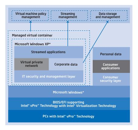
Figure 8. Application streaming. Intel<sup>®</sup> Virtualization Technology supports OS and application streaming, a next-generation standard practice for managing, securing, and delivering applications to users.
