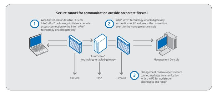
**Figure 3. More secure communication to wired PCs outside the corporate firewall.** An Intel<sup>®</sup> vPro<sup>™</sup> technology-enabled gateway authenticates wired PCs, opens a secure TLS tunnel between the management console and PC, and mediates communication.
