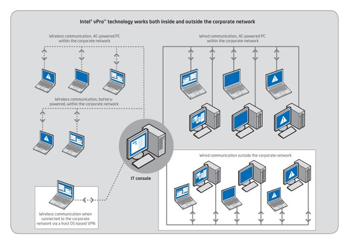
**Figure 2. Remote communication.** Capabilities are available for both wired or wireless notebooks and wired desktop PCs with Intel® vPro™ technology inside the corporate firewall. All capabilities are also available for wired PCs outside the corporate network on an open LAN.<sup>2</sup> Some remote service capabilities for wireless notebooks with Intel vPro technology are also available when the notebook is connected to the corporate network through a host OS-based VPN.
