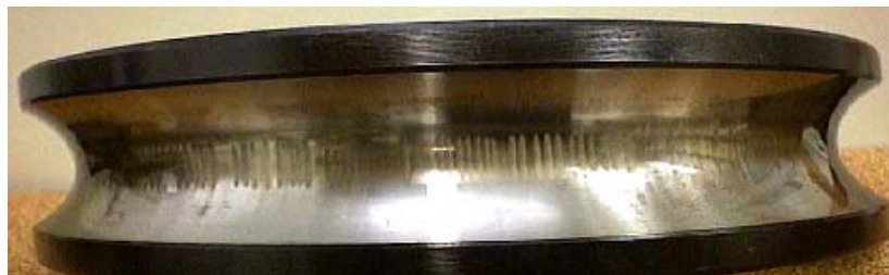
Figure 18 – ‘Characteristic ‘fluting’ wear of inner race
