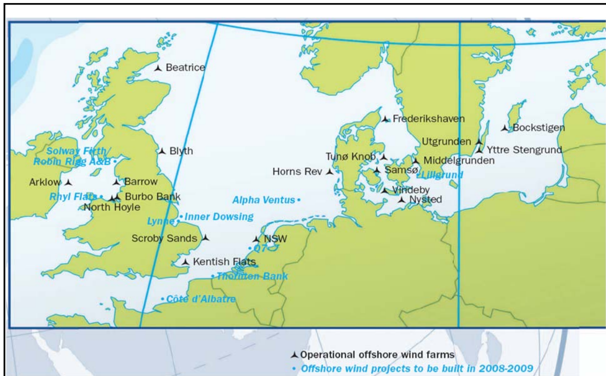
Figure 111 offshore wind farms in Europe and projects to be built in 2009/2010 source: EWEC 2008 1
