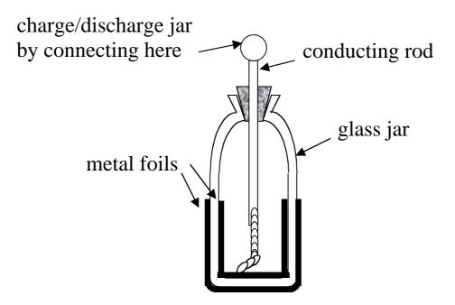
Later experimenters (notably Benjamin Franklin (in 1750s), although many people were interested in 'electricity' at this time) made the first **parallel plate capacitors** using metal sheets separated by glass sheet (window glass!):
