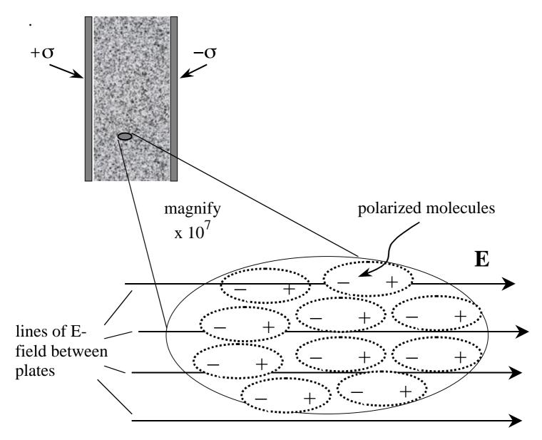
The polarized dielectric has its own 'internal' E-field – in a direction opposite to the 'external field' set up by the capacitor plates. The internal field of the dielectric is that due to the external field.
