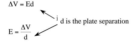
where E is the electric field between plates. The electric field E between the plates is (see end of Section 2.7 (a), this result comes from using Gauss' law)
