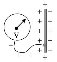
Single charged plate. Charges +Q lead to a potential V. The juxtaposition of like charges – their position relative to one another – brings the plate to potential V, indicated on meter
