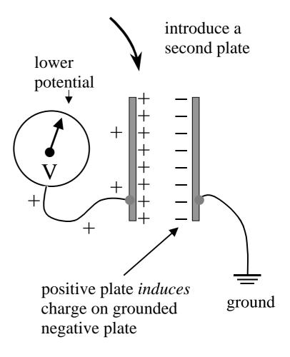
The capcitance of the parallel plate capacitor is easily calculated:
