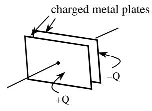
(ii) dielectric material (insulator) between the charged plates:
