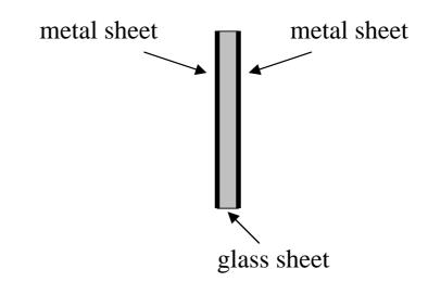
The **parallel plate capacitor** is *the* prototypical capacitor. We consider two versions
