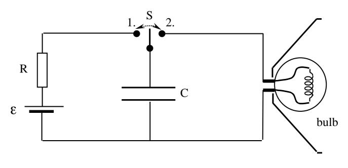
S is a switch. In position 1. it is connected to the battery only and charges the capacitor from the battery which is represented by an emf  $\varepsilon$  in series with the battery's own internal resistance r.
