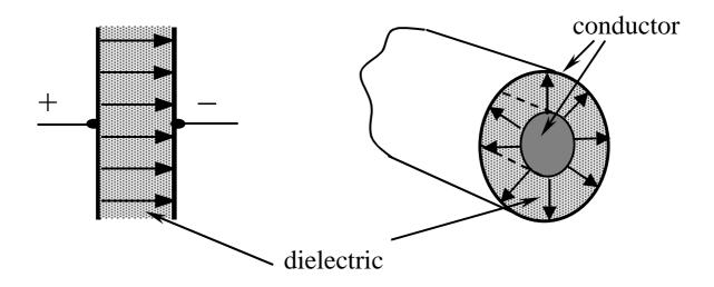
If this electric field is sufficiently strong electrons in the dielectric material are 'ripped' free of their host atoms/molecules. These freed electrons can collide with other electrons in the dielectric material causing them to be released also (a sort of 'chain reaction') and a current can then flow in the dielectric (which was acting as an insulator).
