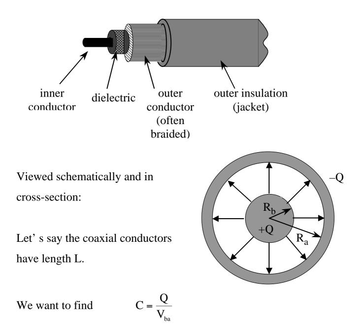
where  $V_{ba}$  is the potential difference between the inner and outer conductor.
