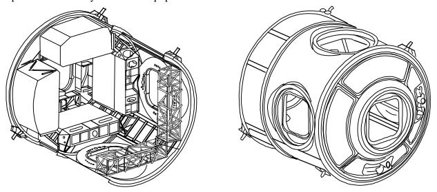
Diagram of interior and exterior views of Unity connecting module
