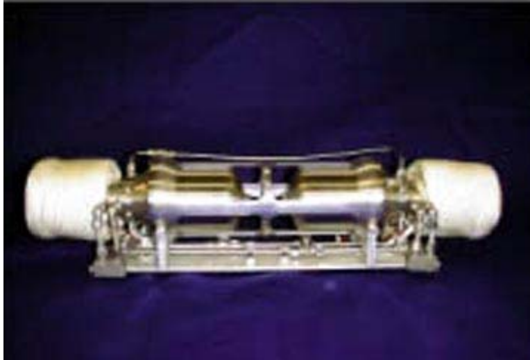
Fig. 19: Stirling engine powered by a radio isotope heat source, NASA Glenn Research Center..
