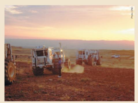
Mertz 18 vibrators were used to acquire 2D seismic in Kurdistan. They all belong to DNO but were operated by Terra Seis International of Canada.
