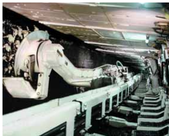
Longwall mining involves the full extraction of coal from a section of the seam using mechanical shearers.
