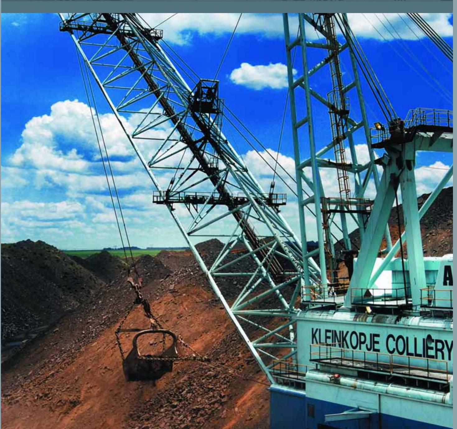
Large opencast mines can cover an area of many square kilometres and use very large pieces of equipment, such as draglines (pictured here). Photograph courtesy of Anglo Coal.
