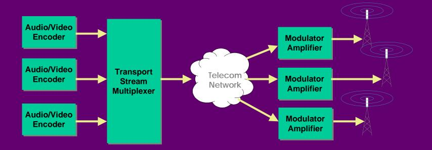
In a DVB-T structure several TV and Radio programs can share a common transmitter network
