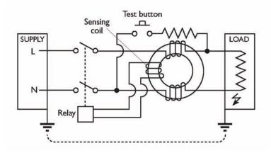
To be effective, the RCD must operate very quickly at a low earth leakage current. Those designed to protect human life are engineered to trip out with an earth leakage current of 30mA within 200mS and at a higher earth current of 150mA, they will trip in less than 40mS. These limits are well inside the safety zone, within which electrocution or fire would not be expected to occur.
