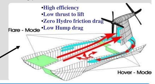
so that air is pushed through the blue channels into the cavity under the body
