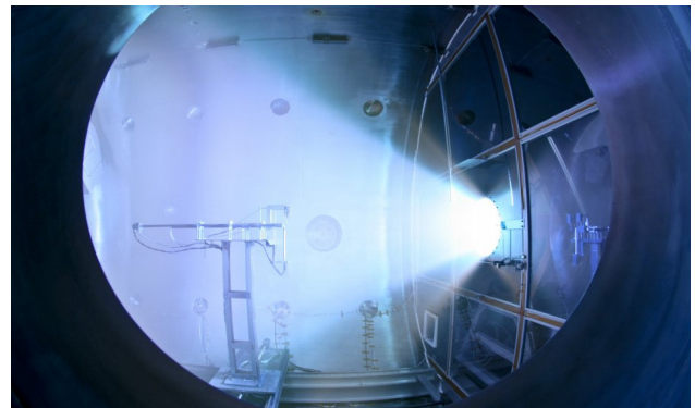
High power VX-200 plasma exhaust is characterized by an array of diagnostics at Ad Astra’s Webster facility.
