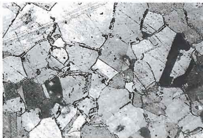
Fig. 7c Solutionized material age-hardened at 500°C for 1 hour (x130)
