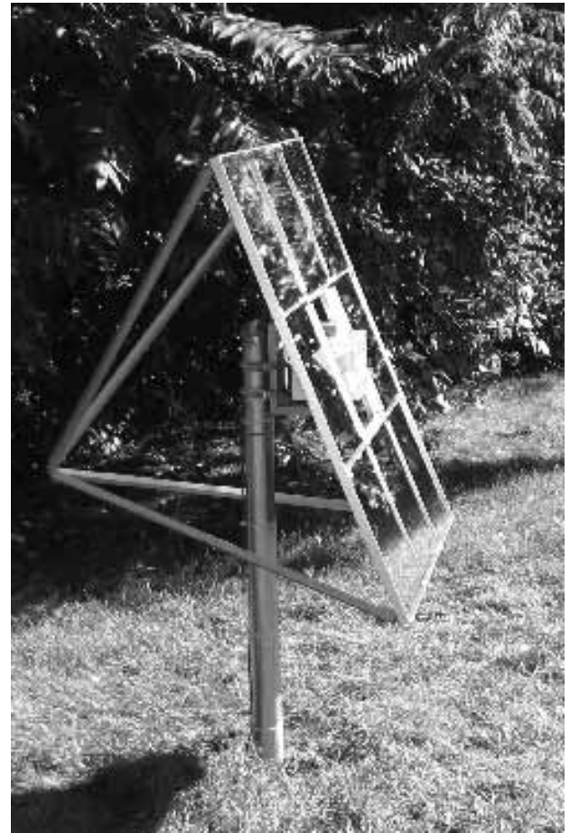
Side view of heliostat shows the stabilizers that strengthen the mirror frame against strong winds.
