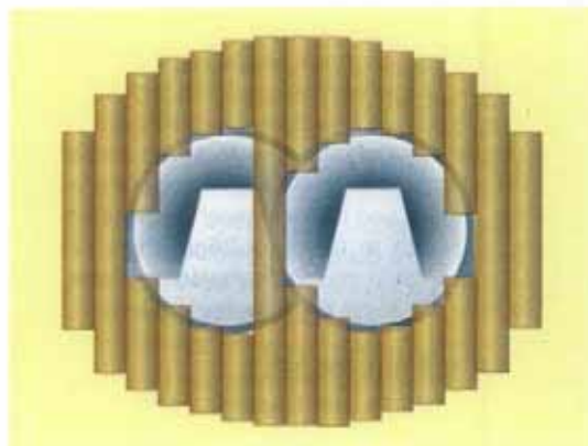
Above: Plan and section of the horizontal jet grouting pattern
