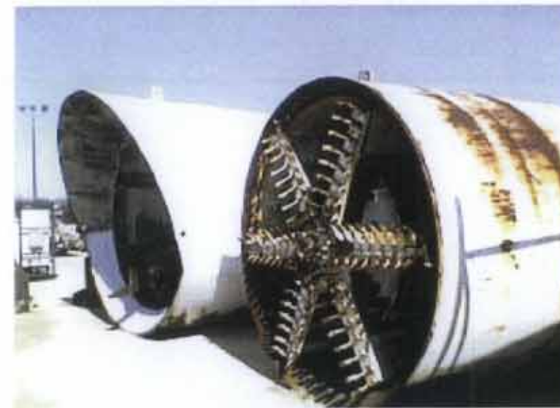
OPEN FACE SHIELD MACHINE WITH ROTARY CUTTER HEAD
