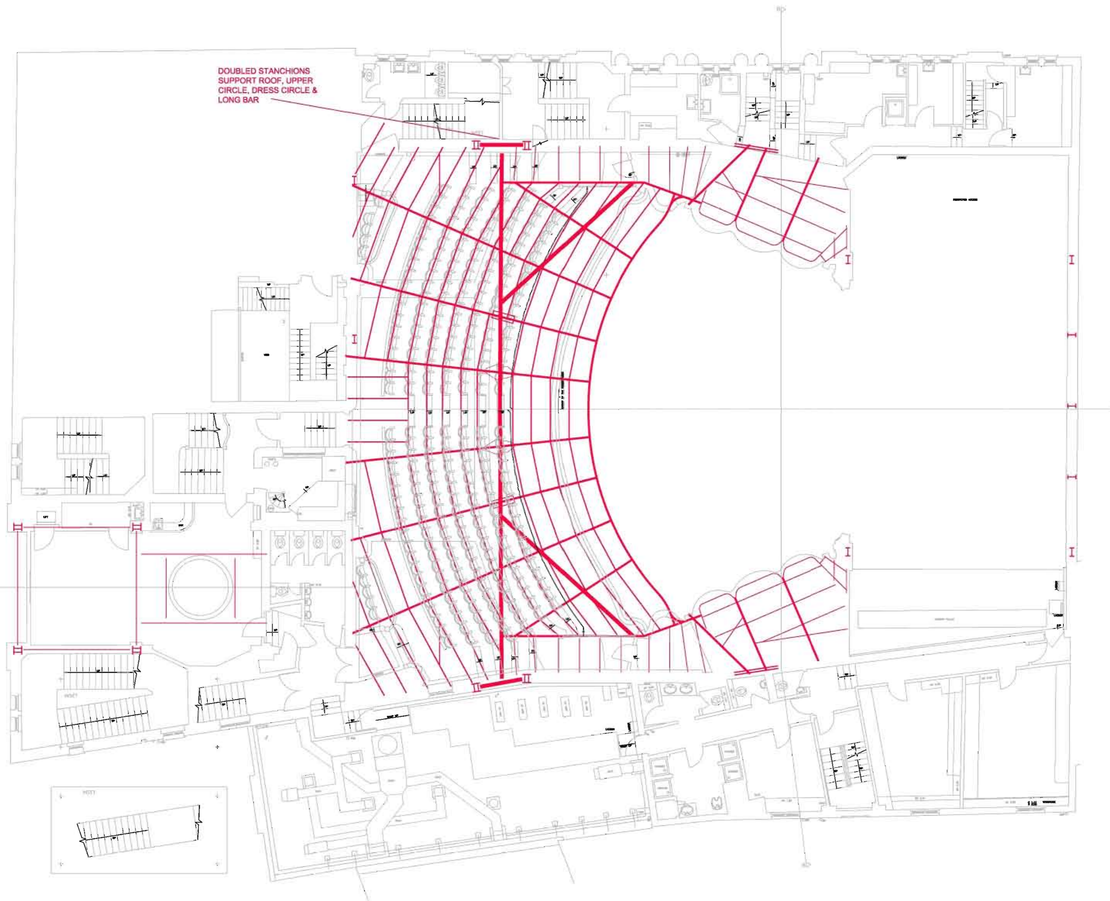
PLAN - SHOWING SECOND FLOOR STEELWORK
