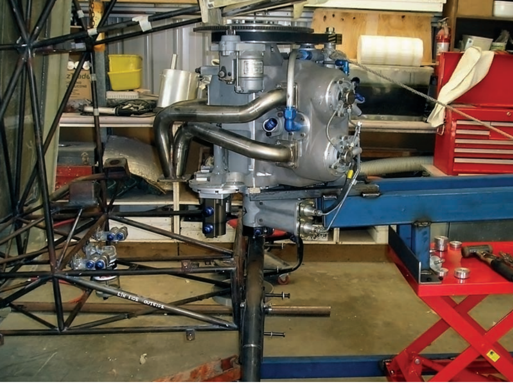
Above, left: The DeltaHawk engine being installed in the airframe. (Pam Johnson) Above, middle: A mock-up of the cooling system layout. (Pam Johnson) Above, right: Assembling body panels. Note the see-through sight gauge in the installed fuel tank. (Pam Johnson)
