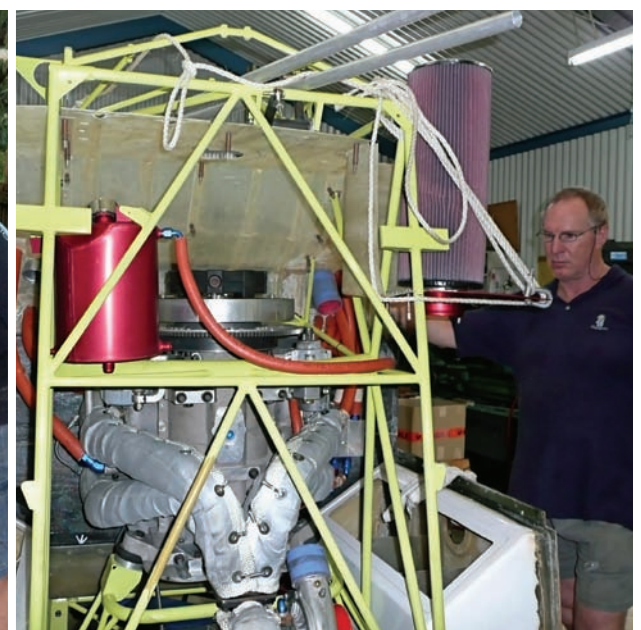
Above, left: Graeme spraying the chrome-moly steel frame. (Pam Johnson) Above, right: Graeme pondering the location of the air filter. (Pam Johnson)
