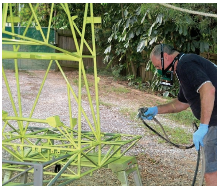
Above, left: Graeme spraying the chrome-moly steel frame. (Pam Johnson) Above, right: Graeme pondering the location of the air filter. (Pam Johnson)
