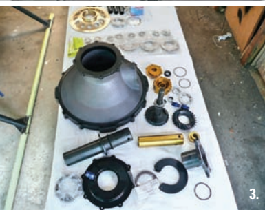
1. Positioning the boom bulkheads in preparation for boom assembly. (Pam Johnson) 2. The DeltaHawk V4 200 hp engine. (DeltaHawk) 3. Main gearbox parts. (Pam Johnson) 4. The main gearbox and swash plate assembled and ready to be installed in the airframe. (Delta Helicopters) 5. Held together with Clecos, the assembled tail boom awaits final riveting. (Pam Johnson)
