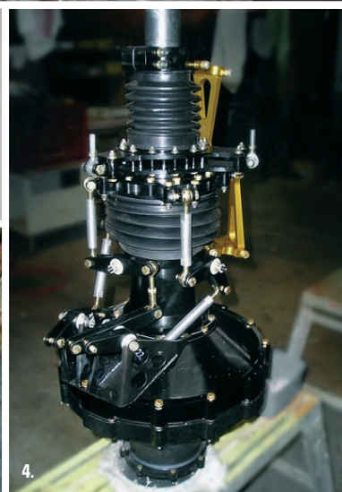
1. Positioning the boom bulkheads in preparation for boom assembly. (Pam Johnson) 2. The DeltaHawk V4 200 hp engine. (DeltaHawk) 3. Main gearbox parts. (Pam Johnson) 4. The main gearbox and swash plate assembled and ready to be installed in the airframe. (Delta Helicopters) 5. Held together with Clecos, the assembled tail boom awaits final riveting. (Pam Johnson)
