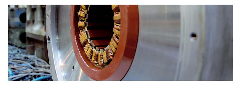
A substantial share of Siemens' current production of compressor trains is fitted with so-called active magnetic bearings (AMB). A glimpse into their concept and performance reveals the appeal of computer-controlled magnetic attraction.
